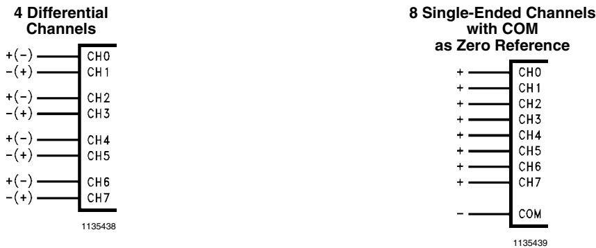
FIGURE 9. Input Multiplexer Options
